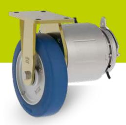
Welded steel heavy duty fixed castor with electric drive and integrated dead man's brake. Wheel with polyurethane tread Blickle Besthane® Soft, with cast iron wheel centre.
