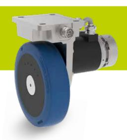
Heavy duty fixed castor with electric drive and integrated dead man's brake. Wheel with Blickle Besthane® Soft polyurethane tread, with synthetic wheel centre.
